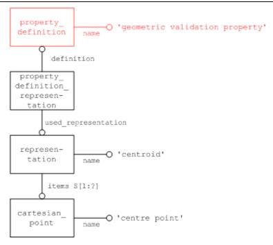
Figure 5: Geometric Validation Property "Centroid"
