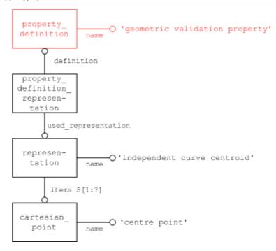
Figure 7: Geometric Validation Property "Independent Curve Centroid"
