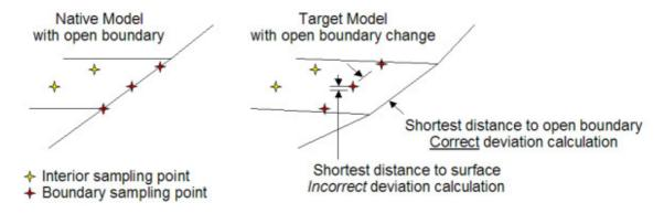
Figure 11: COPS – Sampling Points for an Open Boundary
