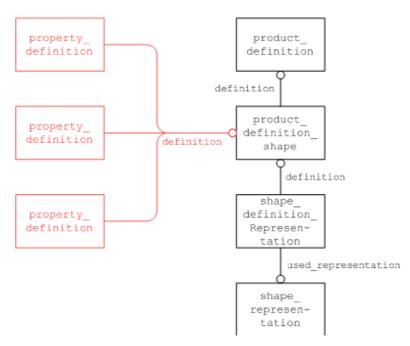
Figure 1: Validation Properties at the Part/Product level
