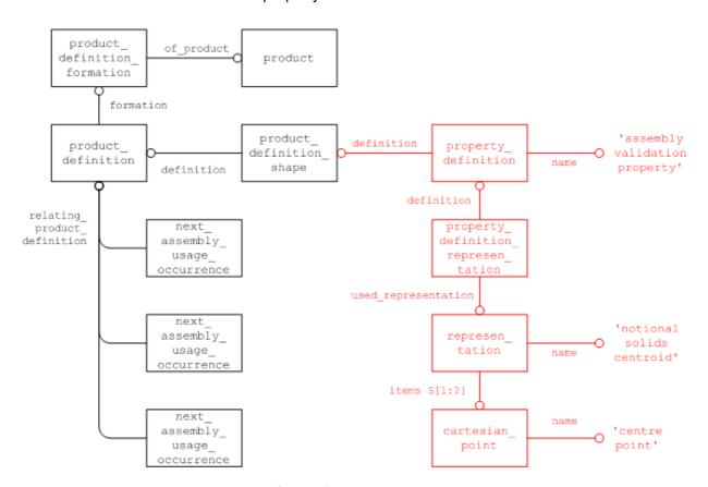
Figure 14: "Notional Solids Centroid Position" Validation Property
