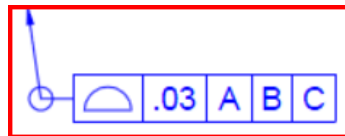
Figure 32: Example Tolerance with All Around Modifier
